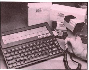
The entire reader weighs only 400g, including cable, and connects directly to the Z88 serial port. Power is supplied from the Ranger rechargeable battery pack, via the Z88, and is sufficient to operate the wand for at least 5 hours' typical use.
