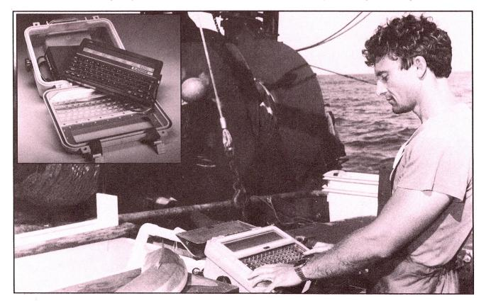
The Hardcase is made from rigid, reinforced plastic which provides resistance to seawater or corrosive atmospheres, and is fully sealed when closed by an integral 'O' ring. The case is in two halves, the top or lid portion retaining the Z88 computer and the bottom or base section the disk drive or other accessories.
