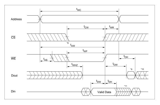
Write Timing Waveform (2) (OE Low Fixed)
