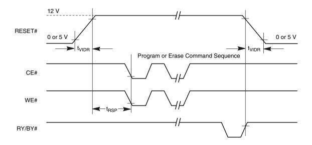
Figure 16. Temporary Sector Group Unprotect Timing Diagram
