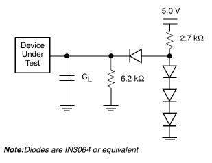
Figure 8. Test Setup
